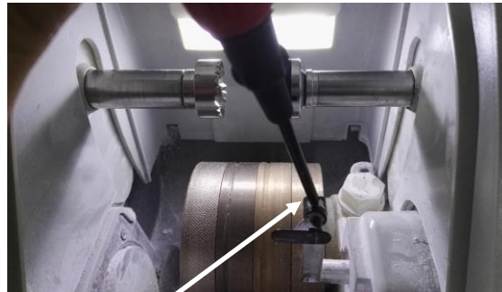
Remove the screws and replace the lens feeler
