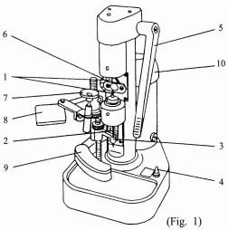
Two drill bits of the same style, drill a lens 1. Drill Bits simultaneously from the upper and lower sides.
