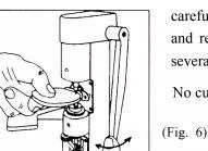
Do not attempt to drill at a sitting but carefully and slowly drill by pushing and releasing the handle alternately several times over. (Fig.6)
