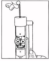
The clearance between the upper drill bit and lower drill bit should be as small as possible, but they must not touch each other. The optimum clearance, push the handle completely, and to adjust it,proceed as follows:
