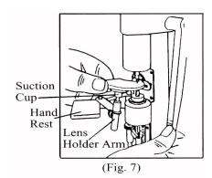
1.Set the lens holder arm onto the hand rest. (Fig.7)
